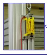
The door is equipped with a safety switch and a mechanical latch.
