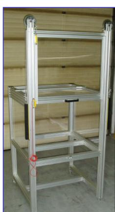
Utilizing our *FrameQuoter* software, FRAME-WORLD designed and built the enclosure pictured at left. The sturdy frame is made of heavy duty 3" x 3" (EX-3) extrusion.
